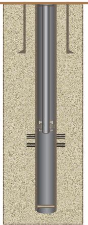
219.1 mm Surface Csg @ 282.0 mKB. Cemented with 20 tonnes TSC  $\,+\,3\%$  LCM  $\,+\,2\%$  CaC12. Cement to surface and 9.0m3 returns.
